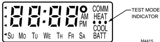
To discontinue the test mode at any time, press the **CLOCK** and **DAY** keys at the same time. The Test Mode Indicators will no longer show on the screen.
